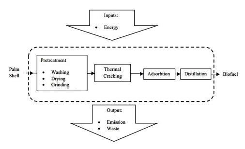
Figure 2. Boundary system of biofuel production process
